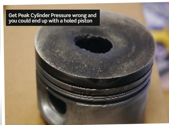
Get Peak Cylinder Pressure wrong and you could end up with a holed piston
