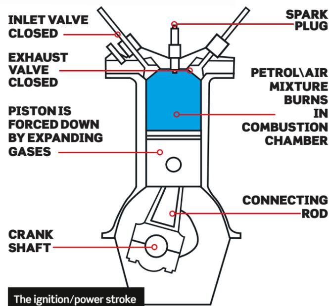
compressed to this immense level, our mixture of fuel and air becomes extremely volatile and a single spark from the spark plug will initiate the combustion of it and release the energy from the mixture, forcing our piston smoothly back down the bore and producing our next stroke — the power stroke.
